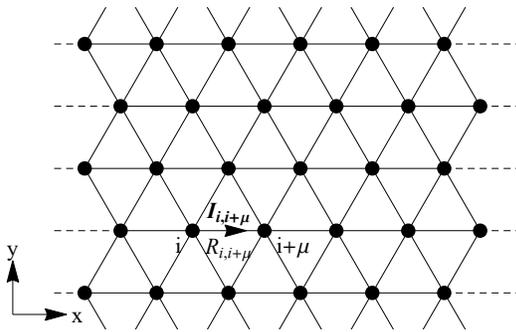
FIG. 4. Triangular lattice of resistors residing on each bond whose resistance  $R_{i,i+\mu}$  is proportional to  $\Delta_{i,i+\mu}^{-1}$ . Sites on the left edge are held at the same potential, and so are those on the right. A potential difference between the edges induces current  $\mathbf{I}_{i,i+\mu}$  which is a vector quantity. The y-direction is periodic, and the dashed lines represent wires with zero resistance.
